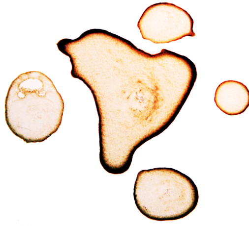
Figure 1.1: The coffee-stain effect demonstrated by tea stains on a desk: when the tea drop has dried, a dark ring of tea particles is left behind.
